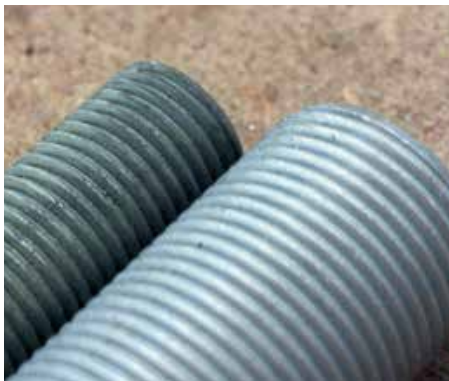
HDG (left) compared with Mechanical Galvanized (right)
