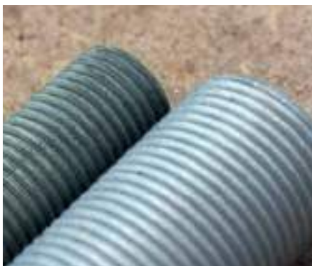
HDG (left) compared with Mechanical Galvanised (right)
