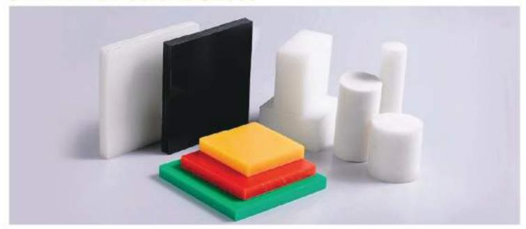
Polyethylene is a semi-crystalline thermoplastic with high toughness and chemical resistance. Polyethylene differs in regards to their molecular weight, which determines the respective physical properties of each grade.
