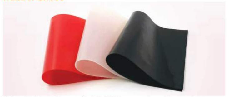
This material provides excellent flexibility across a broad temperature range (-60°C up to +200°C), as it is a synthetic elastomer manufactured from a perfect combination of silicon, carbon, hydrogen, and oxygen. This rubber offers high release properties and performs exceptionally well when exposed to ozone, weathering, and ultraviolet light. It has a good compression set, is highly resistant to moisture and is an excellent electrical insulator.
