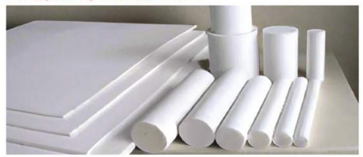
PTFE is a highly crystalline thermoplastic with excellent sliding properties, anti-adhesive surface, excellent insulation properties, an almost universal chemical resistance and an exceptionally broad temperature resistance. However, this is offset by low mechanical strength and high specific weight compared to other plastics.
