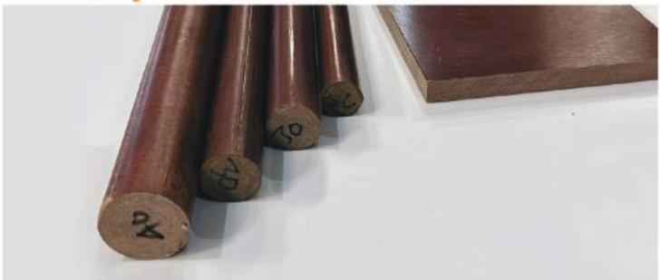
Laminate manufactured from extra fine and super extra fine cotton mesh impregnated with phenolic resin binder, under pressure and heat. This kind of thermoset composite material has proved to be perfect for parts requiring outstanding mechanical strength and electrical properties for machinery, electrometer and electrical appliance. Mechanical grades of fabric reinforced phenolic rods and sheets are available in different grades like:
