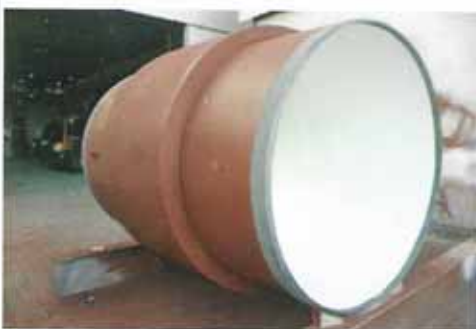
Ø 96" 150# , Gr.B , TP 38 Barg, Monolithic Isolation Joints. Project Riyadh Long Distance Water Transmission System, (RWTS).
