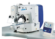
LK-1900S Computer-Controlled, High-Speed, Bartacking Machine
