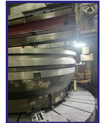
Half Counterweight (Ø4600) Precision boring for large assemblies
