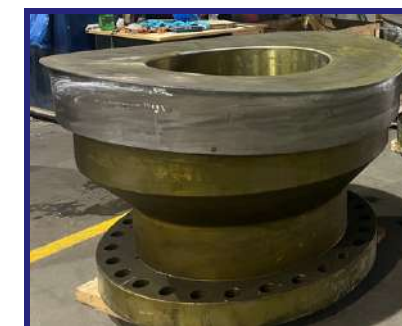
Nozzle Lip Machining CNC rework for re-engineered spares
