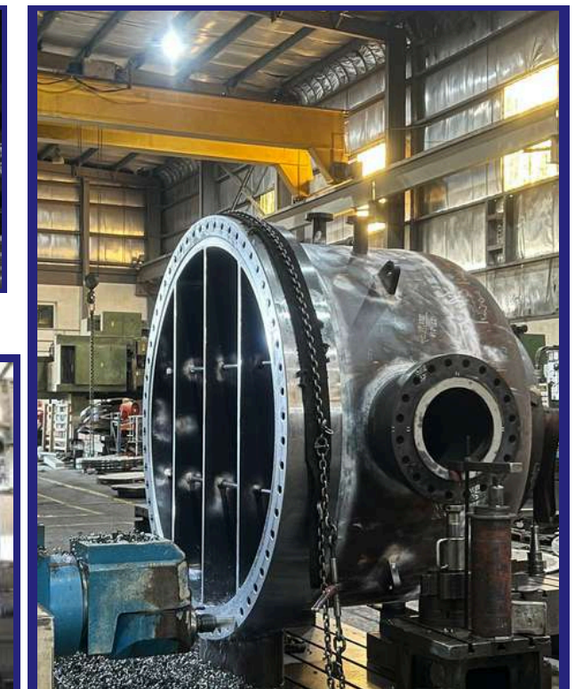
Flanged pipe head (Ø4.2 m) — Oil & gas critical component
