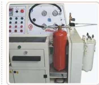
Fire Suppression Hydrostatic Test
