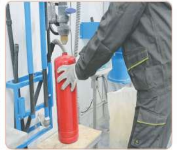
RE FILLING OF FIRE EXTINGUISHER CYLINDER
