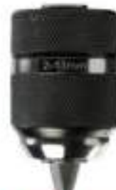
Drill chuck quick connect DIA Ø 2 - 13 mm 1/2\" x 20 UNF connection Keyless IBK.13Q
