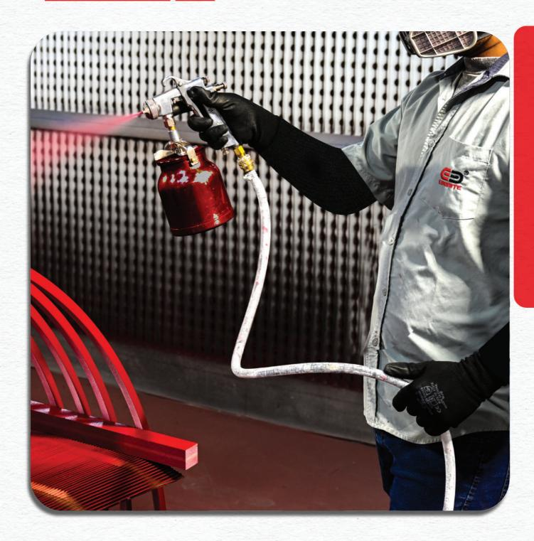
Features specialised booths for various operations. This includes a separate sanding booth equipped with an integrated dust collection system, manual primer and final spray booths, an automatic spray line, and an additional booth featuring the latest artificially accelerated paint drying technology.
