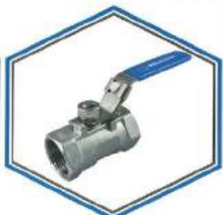
SS 1-Piece Ball Valve Reduced Bore 1000 WOG NPT Body: CF8M/ Ss316 Size: 1/2" to 2"
