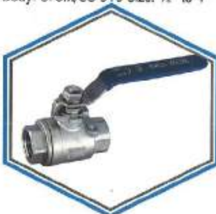
SS 2- Piece Ball Valve Full Port 1000/3000/6000 WOG NPT Body: CF8M/SS 316 Size: 1/2" to 4"
