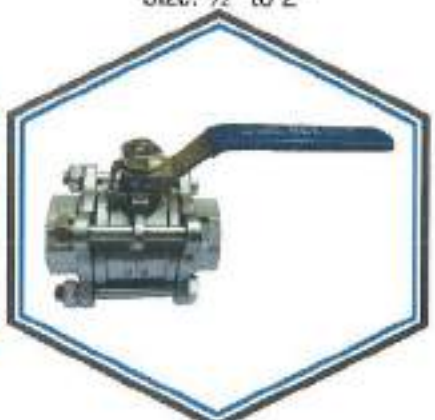
SS 3-Pice Ball Valve Full Port 1000/3000/6000 WOG NPT Socket Weld Body: CF8M/SS 316 Size: 1/2" to 4"
