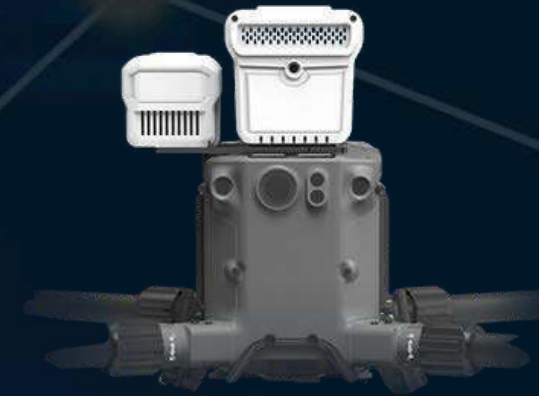
Sniffer4D 1ppm NDIR CO2 Sensing + Sniffer4D MP-TDLAS Methane Sensing
