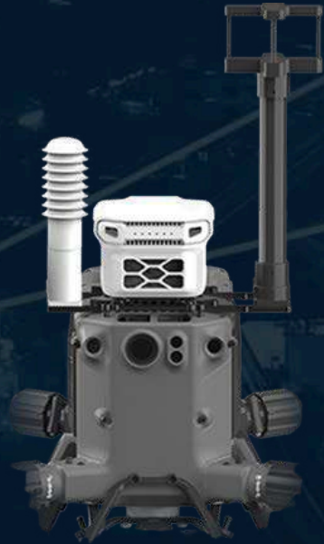
Sniffer 4D Mini2 Multi-gas Sensing + Wind Sensing + External Temperature & Humidity Sensing
