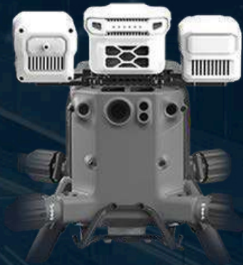
Sniffer 4D Mini2 Multi-gas Sensing + Sniffer4D MP-TDLAS Methane Sensing + Sniffer4D 1ppm NDIR CO2 Sensing
