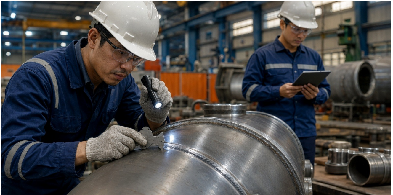
Visual weld examination and dimensional verification in a controlled fabrication environment
