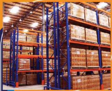
SELECTIVE PALLET RACKING
