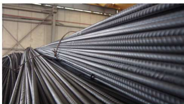
Reinforcement steel bars
