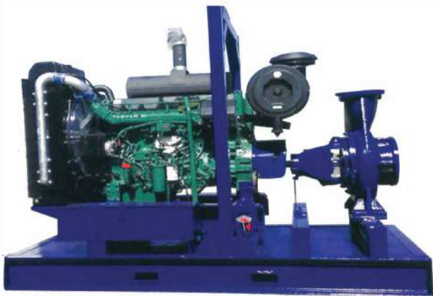
Pump : Lubi-end Suction Head : 70 Mtr Engine: TAD 943-VE-Volvo Penta Suction / Discharge Flow : 1180 Mtr. Cube/Hr - 10" / 12"
