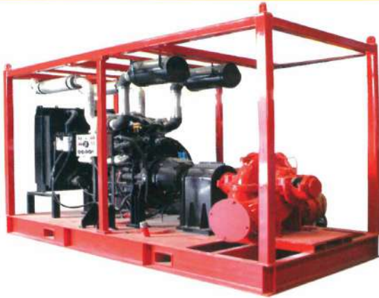
Pump : ACP-250-D Head : 120 Mtr Engine: 16-V-92 Detroit Suction / Discharge Flow : 1200 Mtr. Cube/Hr - 10" / 12"
