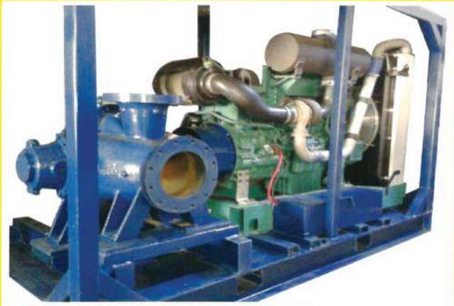
Pump : Mattar & Platt-Split Case Head : 120 Mtr Engine: 1643-VE-Volvo Penta Suction / Discharge Flow : 1200 Mtr. Cube/Hr - 10" / 12"
