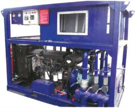
Unit : Hydraulic Flushing Rig Pressure : 70 Bar Engine: Perkins Discharge Flow : 1000 LPM - 3" / 2" NPT
