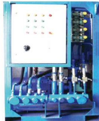
Unit : Test Powe Pack Pressure : 350 Bar Motor: Weg Discharge Flow : 100 LPM - 1" NPT
