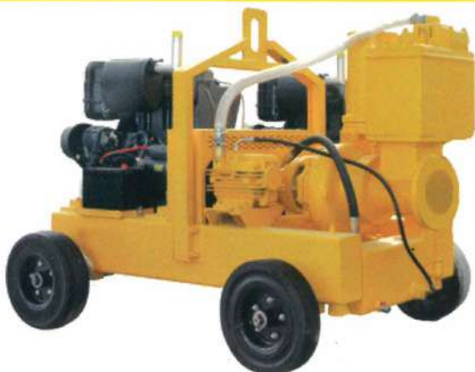
Pump : Dewatering Head : 40 Mtr Engine: Kirloskar / Dutz Suction / Discharge Flow : 350 Mtr. Cube/Hr - 6" / 5"
