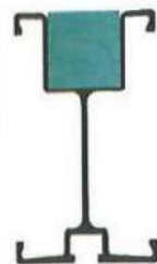
140 – H BEAM w/ WOOD (For Joist)
