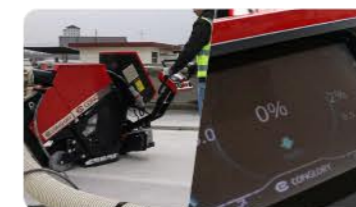
Abrasive flow controlled by Digisteer
