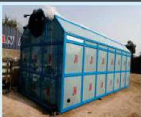
Fauji Food limited Bhalwal, 10 TPH boiler Body
