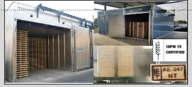
During the process of Heat Treatment, pallets are placed in a special chamber and heated according to a specific criterion. In order to be ISPM 15 compliant, a wood core temperature of 56°C/133°F must be reached and maintained for a period of 30 minutes or more.
