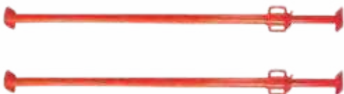
Shuttering Props Weight : 10 kgs. / pcs. | Max. Length : 3.9m Min. Length : 2.2m | Adjustable Length : 125mm Number of Pin Hole : 12 | Safety Load When Closed : 1.7 mt
