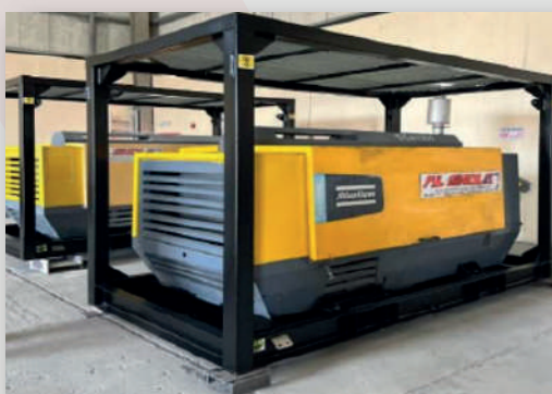
LIFTING FRAME STRUCTURE AS PER DNV STANDARD
