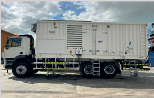
Truck Mounted Mobile Enclosure for 625kVA VolvoPenta Genset; Noise Level 70dB @ 10 mtr
