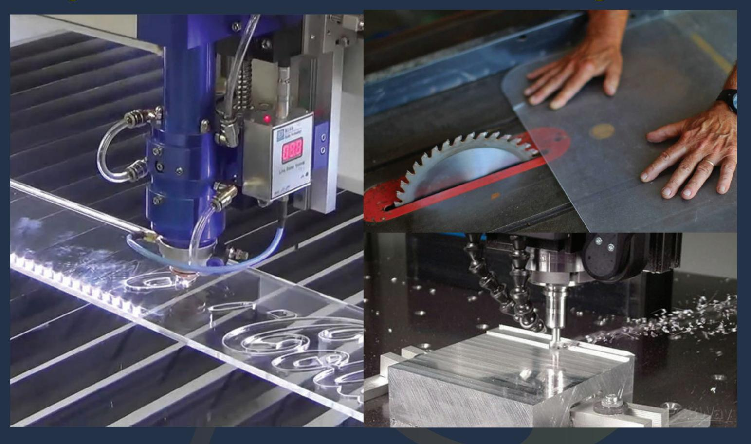
Laser cutting is a process of cutting forms or designs into sheet metal or other structural materials that is most commonly employed in the manufacturing business, but it is also gaining favour in other sectors such as schools and hobbyists. A precise method of cutting a specific pattern from acrylic material using a CAD file as a guide. In other terms, it is a digital subtractive creative approach that uses a laser to cut or engrave a specific material.
