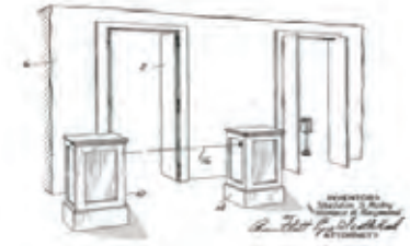
1931: STANLEY patents the world's 1st hands-free door operator actuated by photo-electric cells.
