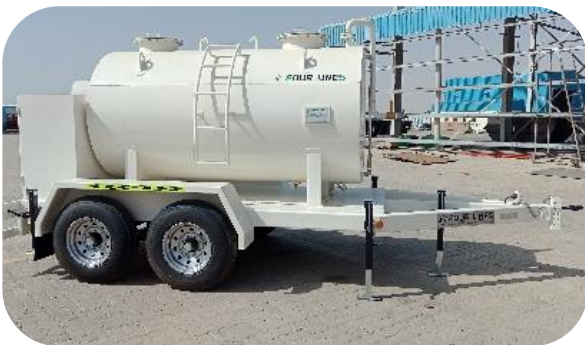
3000 LTR FUEL TANK ON TOWING TRAILER
