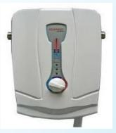
Instantaneous inline water heaters are small electrically powered units that heat water 'instantly' as it flows through the product. Instantaneous water heaters are compact, will not run out of hot water and have no stand-by energy losses but have to be wired to the electric consumer unit.
