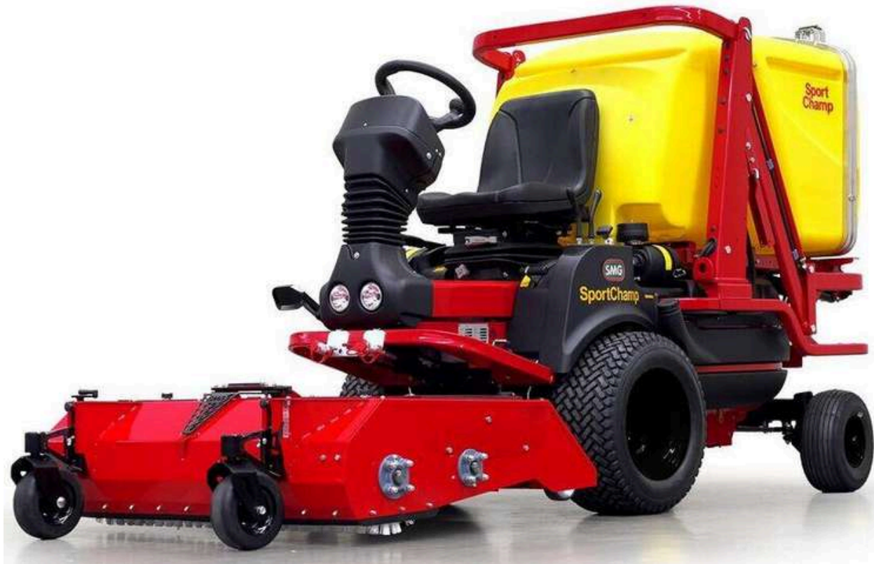
SC3D4HL-Multifunctional ride-on machine for contractors for the advanced maintenance of artificial turf.
