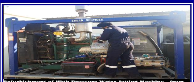
efurbishment of High Pressure Water Jetting Machine from
