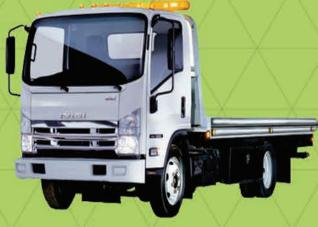
We also provide recovery vehicle. The entire back to these truckis fitted with a bed that can be hydraulically inclined and moved to ground level allowing the vehicle bieng tower to be placed and its under its own power or pulled by a winch
