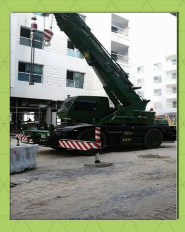
Our rough terrain cranes are used off-road in building bridges, at industrial plants and heavy construction , these cranes are hydraulic, self-propelled mounted on an undercarriage. These cranes are normally transported by a truck or lowbed trailer. Our Fleet includes these cranes manufacture by Tadano, Kato and Grove etc.
