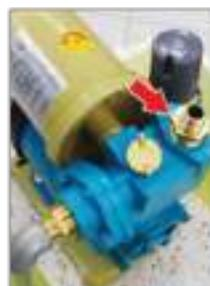
3. Install another outer pump connector on the outlet of the pump.
