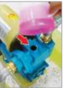
5. Unscrew the water injecting nozzle and fill it with water.
