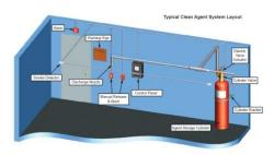
through heat absorption, leaving no residue, thus minimizing downtime after a fire and making FM-200 suppression systems accepted and respected worldwide with over one hundred thousand installations in more than seventy countries.
