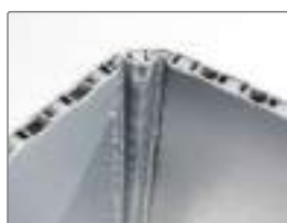
Honeycomb structure of the container wall
