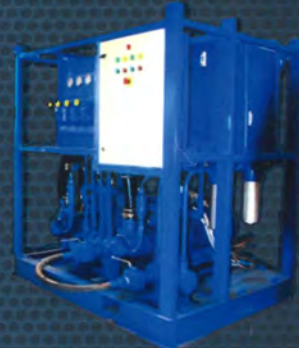
Hot Oil Flushing / Pressure Testing
