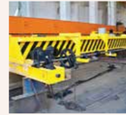
Manual Operated Overhead ( From 100Kg to 5Ton capacity )
