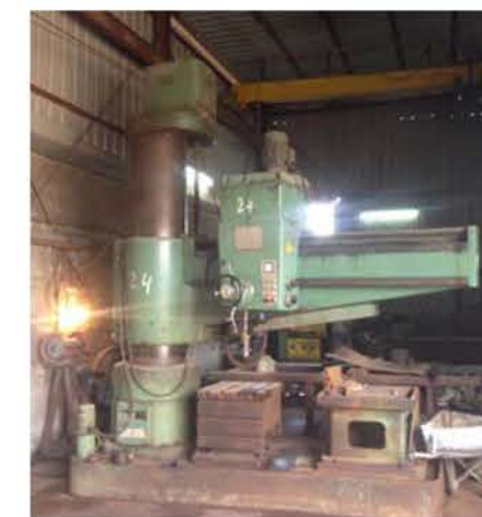
Radial Drilling Machine Capacity 3000mm @ 100mm
