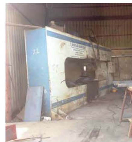
Steel flanging machine Capacity 4000mm Dia, 25mm thickness
