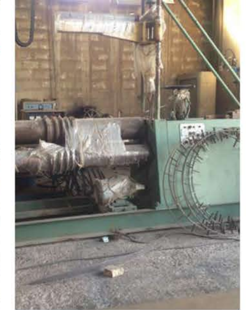
Plate rolling machine Capacity 2000mm @18 mm
