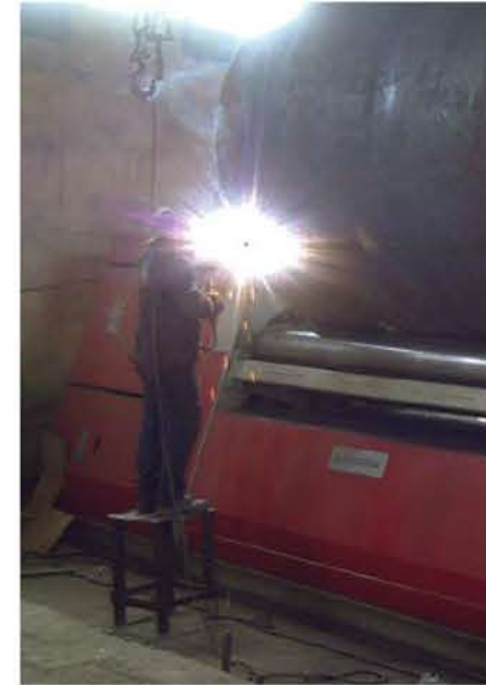
Plate rolling machine- AKYAPAK -Turkey Capacity 3000mm @ 30mm
