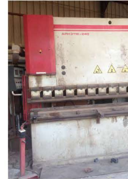
Sheet bending machine - Baykal-Turkey Capacity 240 Ton
