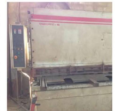
Sheet metal cutting machine - Turkey Baykal - 3000mm length, 12 mm thick
