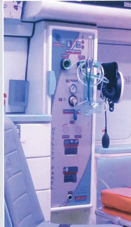
Utility Panel contains O2 flow meters, O2 cylinder changeover switch, Pulse Oximeter & etc.
