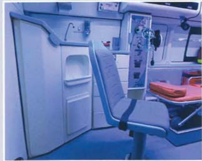
ABS/GRP molded cabinry with lock & key and customized revolving seat.
