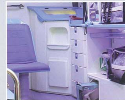
ABS/GRP molded cabinetry with lock & key and door lights
