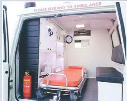
Utility Panel contains O2 flow meters, O2 cylinder changeover switch, central suction control & etc.
