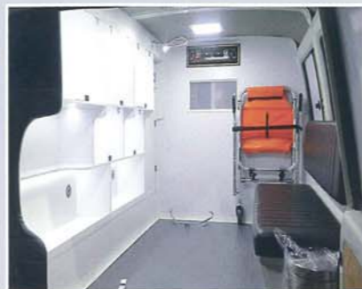
Side & overhead cabinetry sufficiently accommodate all equipment.
