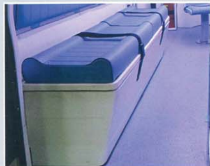
Side Bench can accommodate an extra patient and has underneath storage for folding stretcher & other items.
