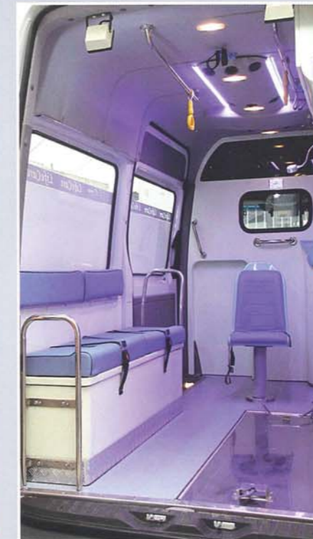
Side Bench can also accommodate an extra patient & have storage beneath, stretcher area reinforced with S/S sheet.
