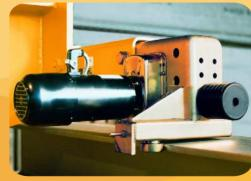
systems and trolleys are equipped by default with high-strength polymer wheels. In comparison with steel wheels, these wheels run particularly quiet and provide significantly improved friction values, preventing slipping and spinning of wheels. The reduced slip between wheel and rails greatly reduces wear on both components and minimises noise as well.
