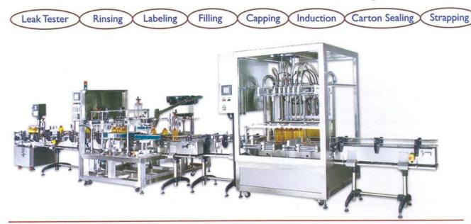
LEAK TESTER: designed for plastic bottles/containers leak testing. Specially for bottle makers, soft drinks, motor oil, lubricants, detergent and chemical industries to ensure bottle quality before liquid filling.
