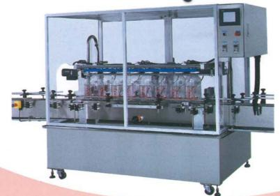
FILLING STATION. Fast change-over design for different size of bottle, Mitsubishi PLC Control System (Japan made), wide range of Filling, driven by AC motor individually, No bottle - No filling safety device, Photocell sensors (Germany SICK brand). Machine construction covered by SUS# 304.
