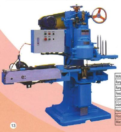
S-C3A(L) sanitary Seamer modified from model SC3(L) can body feeding path from S type change to staraight feeding. Timing spiral feeding device and sensor for INC NC control made it more easy to connect with liquid filler. Suitable for wide range round cans seaming and simple or can size change over. adjusting, maintenance, and surprising in the quality and stability of the soaming offect, S-CA(L) Seamer win a reputatino of mid-speed can seamer.
