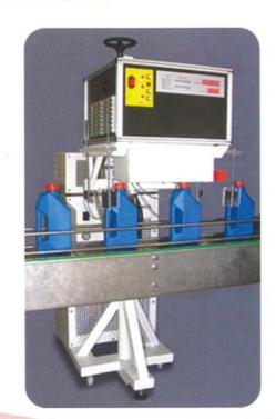
**LABELING STATION:** designed for I flat / oval /around shape bottles and containers.
