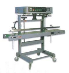
Specifications: Horizontal & Vertical type for handling different sizes . Adjustable conveyors with different load capacity.
