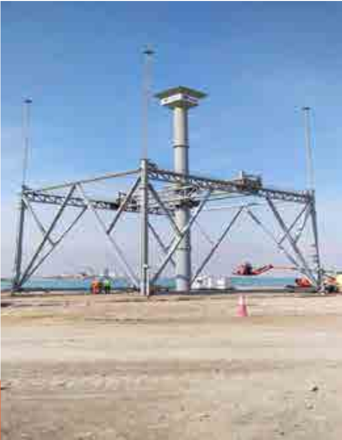
Specification: (Gantry crane for marine application) 4 Nos of Hydraulic cylinder with load capacity of 80 M Tons with double pilot check valve for safety.
