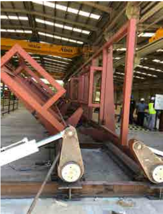
Specification: (Hydraulic Tilting Table) 2 Nos of Hydraulic cylinder with load capacity of 75 M Tons with double pilot check valve for safety.
