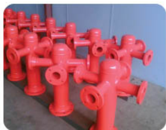
PROJECT: TAKREER - UMM AL NAR REFINARY - WATER INTAKE 300 MM DIA PIPE SPOOL THERMOPLASTIC (PVC) POWDER COATING (INTERNALLY & EXTERNALLY) - 450 MICRON
