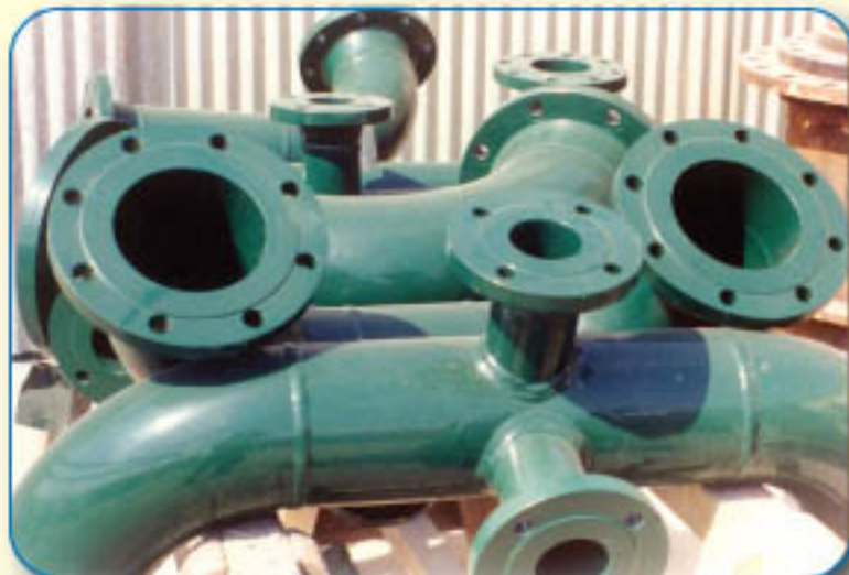
PROJECT: TAKREER - UMM AL NAR REFINARY - WATER INTAKE 300 MM DIA PIPE SPOOL THERMOPLASTIC (PVC) POWDER COATING (INTERNALLY & EXTERNALLY) - 450 MICRON
