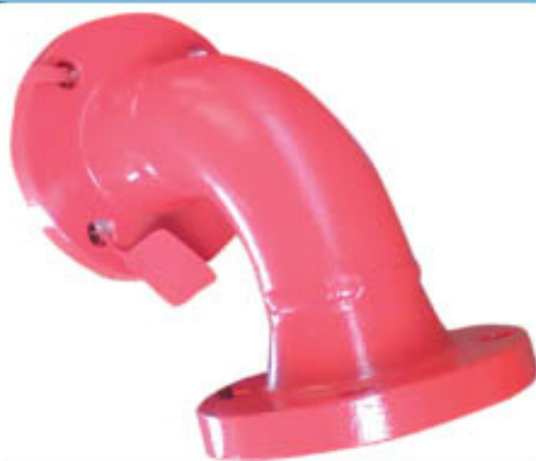
PROJECT: TAKREER - UMM AL NAR REFINARY - WATER INTAKE 300 MM DIA PIPE SPOOL THERMOPLASTIC (PVC) POWDER COATING (INTERNALLY & EXTERNALLY) - 450 MICRON
