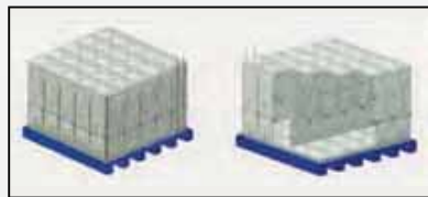
3D Model of GRP Tank with Inner Partition
