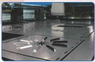
Turret Punching is a form of metal processing by punching operation of the sheet material. This process is well suited for mass production of typical sheet components. It is also very fast and economical compared to Laser or Water Jet Cutting method but the initial tooling cost is relatively high. We have capacity to handle sheets measuring up to 3 m long and 1.5 m wide with a punching capacity up to 23 Ton.
