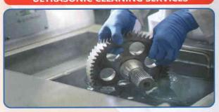
Ultrasonic cleaning is a process that uses ultrasound to agitate a fluid. Ultrasonic cleaners are used to clean many different types of objects, such as tools, car fuel injectors & industrial machine parts. We are capable to handle parts up to 1.15 x 0.5 x 0.45 m overall size weighing up to 350 kg.
