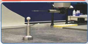
A coordinate measuring machine is a device that measures the geometry of physical objects by sensing discrete points on the surface of the object with a probe. We have possibility to measure parts up to 2.0 x 1.2 x 1.0 m size which greatly helps us in measuring complicated and otherwise difficult to measure part geometry.
