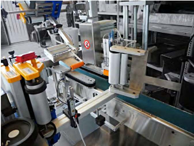
Special labelling system with three labelling heads is designed for application of front, back and security label on cylindrical, rectangular and hexagonal bottles and jars.
