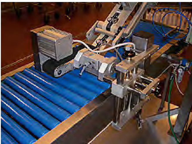
(horizontal roller) applies labels on containers of cylindrical shape. The “Pharma” version is for labelling of ampoules or vials. The “Industry” version is for labelling batteries or cylindrical cartridges.
