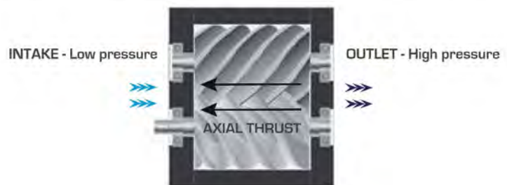
Fig. 4 - The intake and outlet ports are set at opposite ends of the compressor in the axial direction, giving rise to an unbalanced pressure profile along the compressor length
