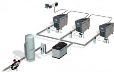
Compressed Air System
