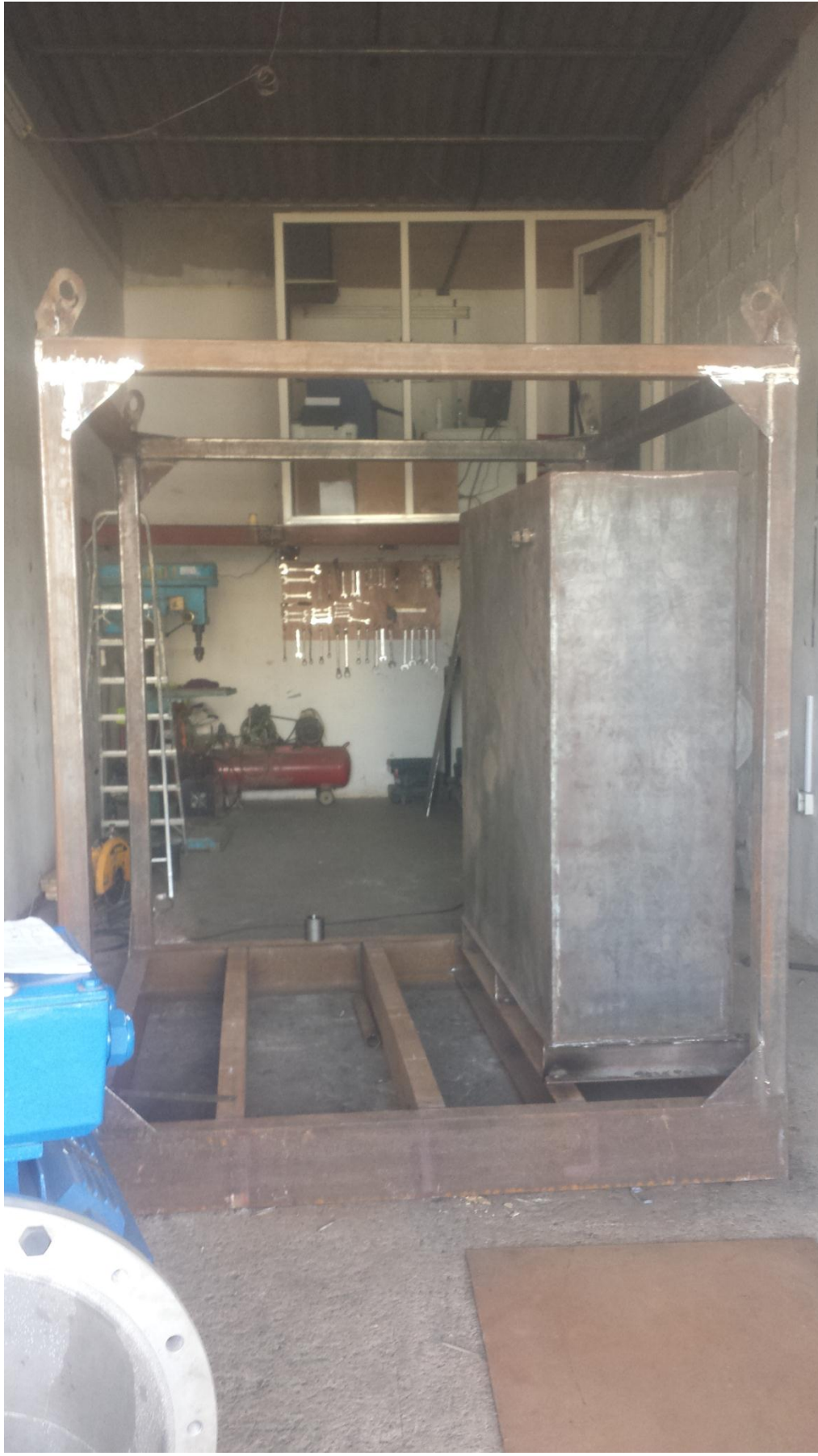
TANK WITH SKID
