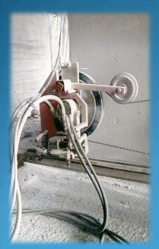
We can cut concrete columns, beams, slabs as well as stairs etc. of different depths using concrete diamond wire. With Concrete wire Cutter we cut concrete up to the infinite depth. This machine is operated through remote control and having a wide range of safety system. The heads of both the machines: Saw Cutter and Wire Saw Cutter are changed. Rest of the unit remains same.
