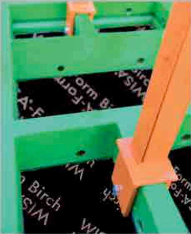
Bolts or pins are also connect the upper and lower pivot with the panel
