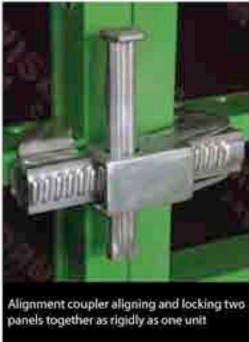
Standard panel connection. Typically only 2 to 3 couplers are required for 2.7m | 8' 10.75" height
