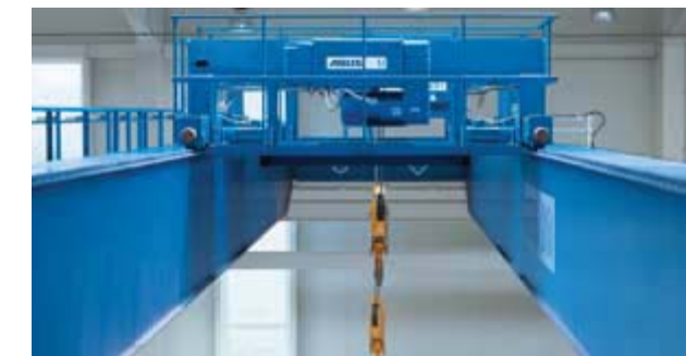
This ABUS type DB electric wire rope hoist has a walkable service platform for even easier maintenance (Rösta).
