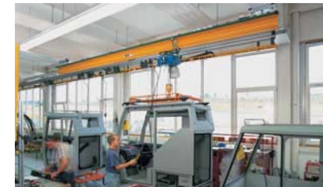
Linear point-to-point handling of vehicle cabs using the ABUS ESB monorail system (Liebherr, Ehingen)
