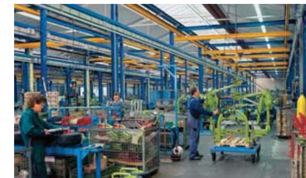
An ABUS EHB single-girder crane ensures optimum material flow on a combine harvester production line (Claas).
