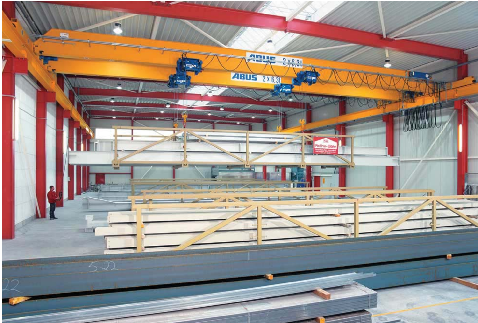
Four synchronized type E electric wire rope hoists handling loading racks for steel structures (Krähe + Wöhr).
