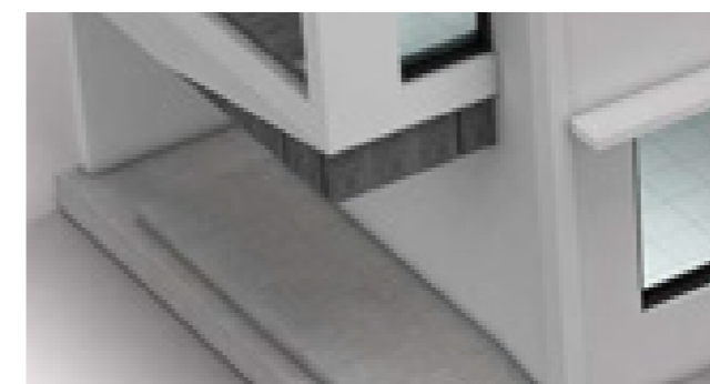
Soffit Insulation Suggested Product: STYRO Graypor 220
