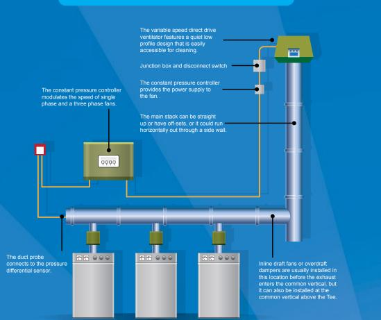
The Chimney Automation System is a demand controlled exhaust system designed for commercial boilers and water heaters in buildings where the exhaust is powered by a chimney fan on the exterior of the building. It maintains a precise draft by constantly adjusting the exhaust rate to meet current needs. The concept can provide substantial operating savings over gravity systems and other significantly better draft control which reduces emissions.
